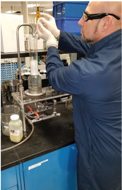
Testing of a defoamer in a surfactant foaming media
