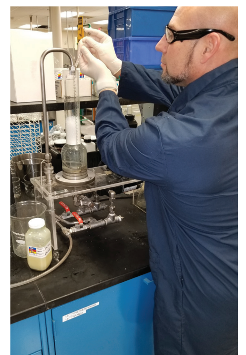
Testing of a defoamer in a surfactant foaming media
