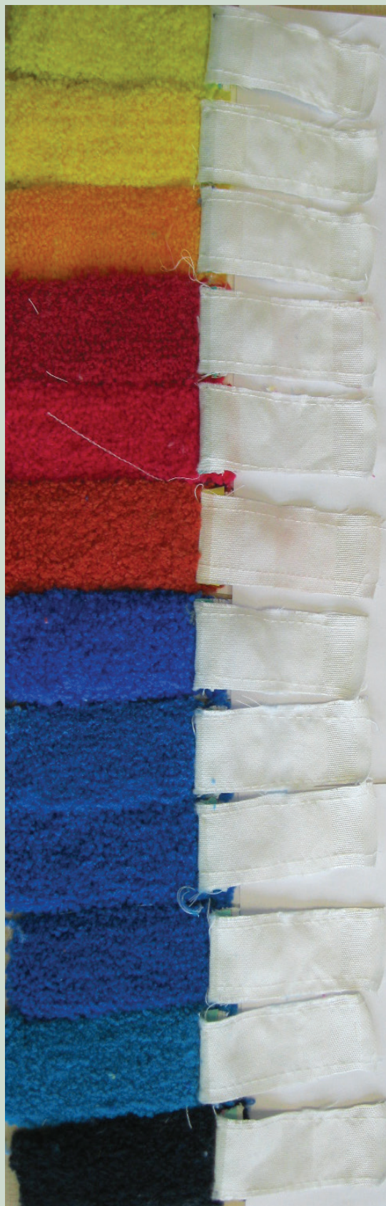
Water fastness severe (ISO 105-E01)
