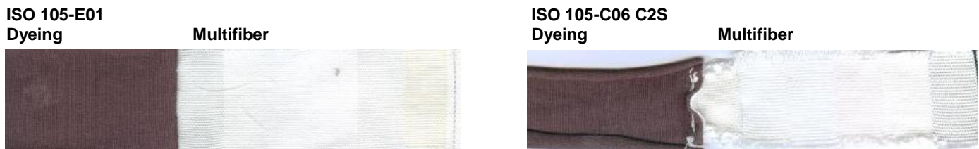
Figure 3: Fastness test to water severe (ISO 105-E01) and fastness to washing by 60°C (ISO 105-C06 C2S)
